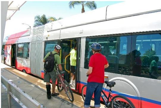
Omnitrans began offering bike racks on buses in 1996. The original version held two bikes. Due to growing demand, Omnitrans began transitioning to 3-bike racks in 2012. Racks are on the front of Omnitrans 40-foot buses and OmniGo vehicles. The sbX rapid transit line can hold up to four bikes inside the rear section of its 60-foot articulated coaches.
