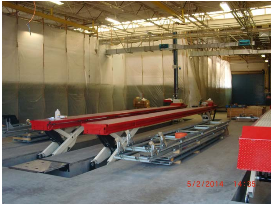
3. New platform bus lifts installed in Maintenance Facility (Building A)
