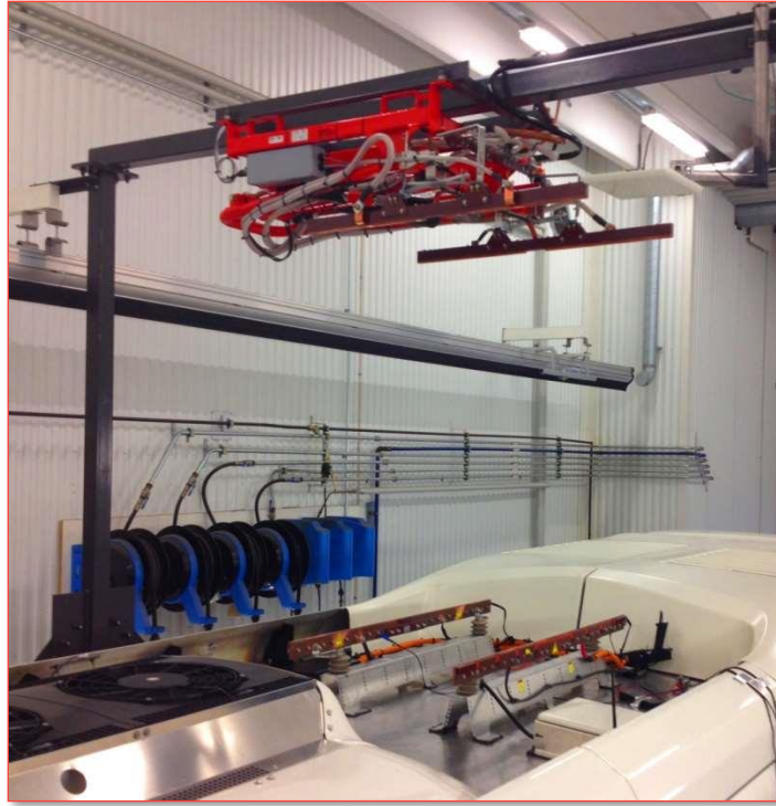
Figure 4-2. Inverted Pantograph and Charge Rails
