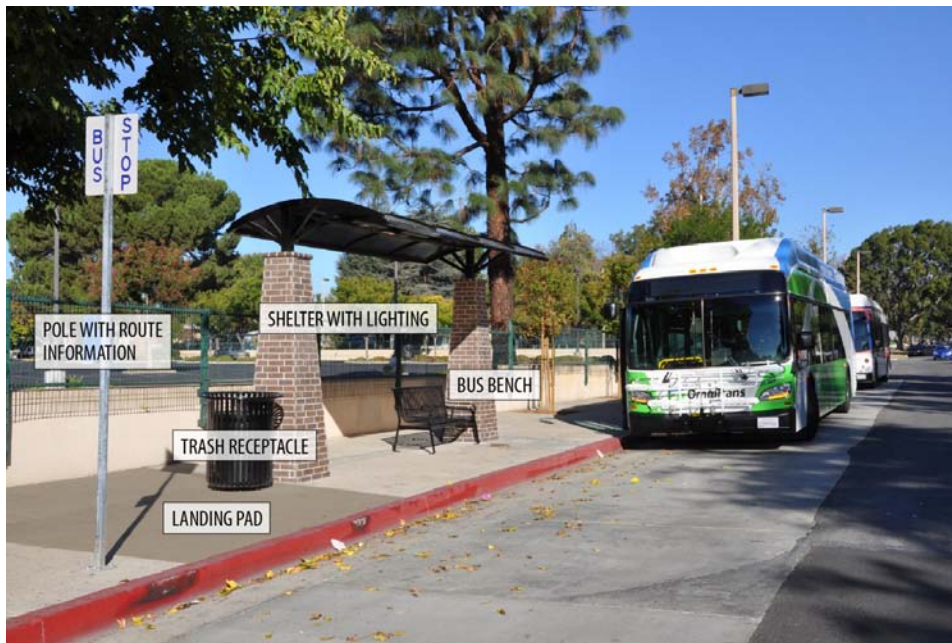
Figure 3-4: Standard Omnitrans Local Bus Stop
