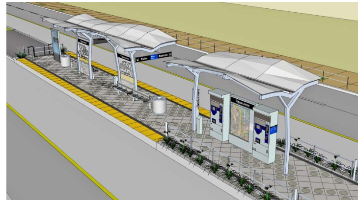
Figure 9-12: Structural columns and undulating roof shelter
