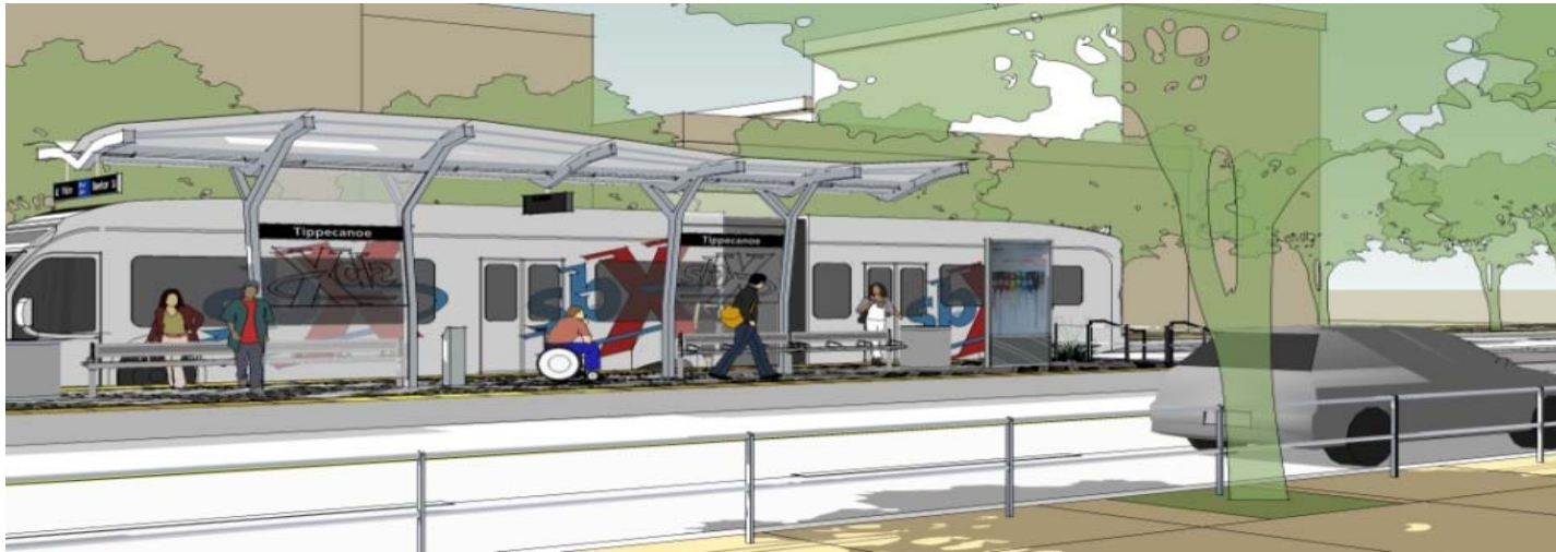
Figure 9-7: Railings or low fences or planters direct pedestrians to cross in the legal crosswalk to the platform
