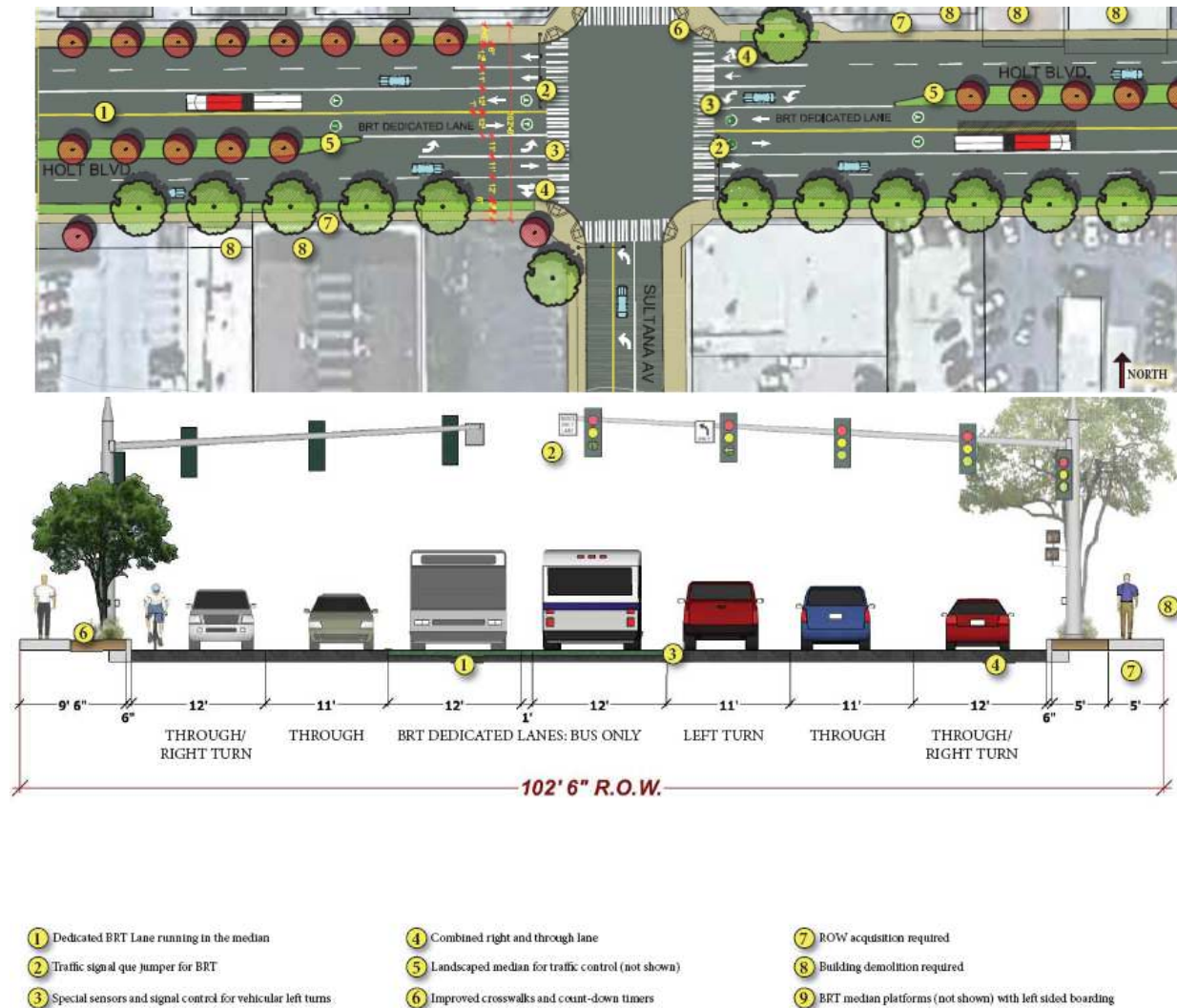
Figure 10-3: Example of a street cross section for dedicated median lane BRT
