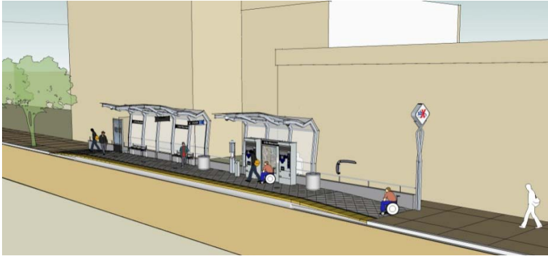
Figure 9-5: Accessible sloped walk and curb height at station platform
