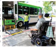
the vehicle with a mobility device, it is a best practice to back your device onto the lift and then into the vehicle.
