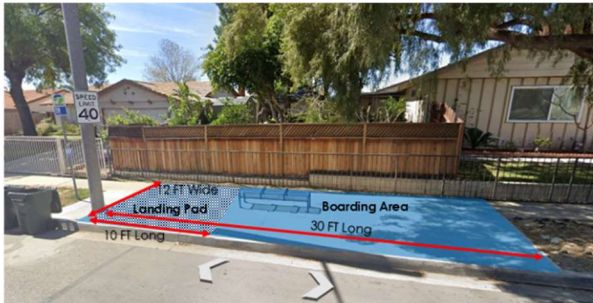
BASIC: Meets all the requirements and has a bench as a basic amenity.
