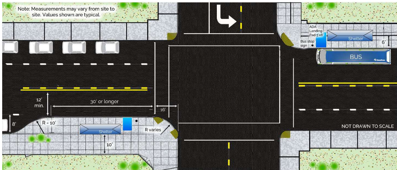
Figure 5-8: Extended curb installed at intersection.
