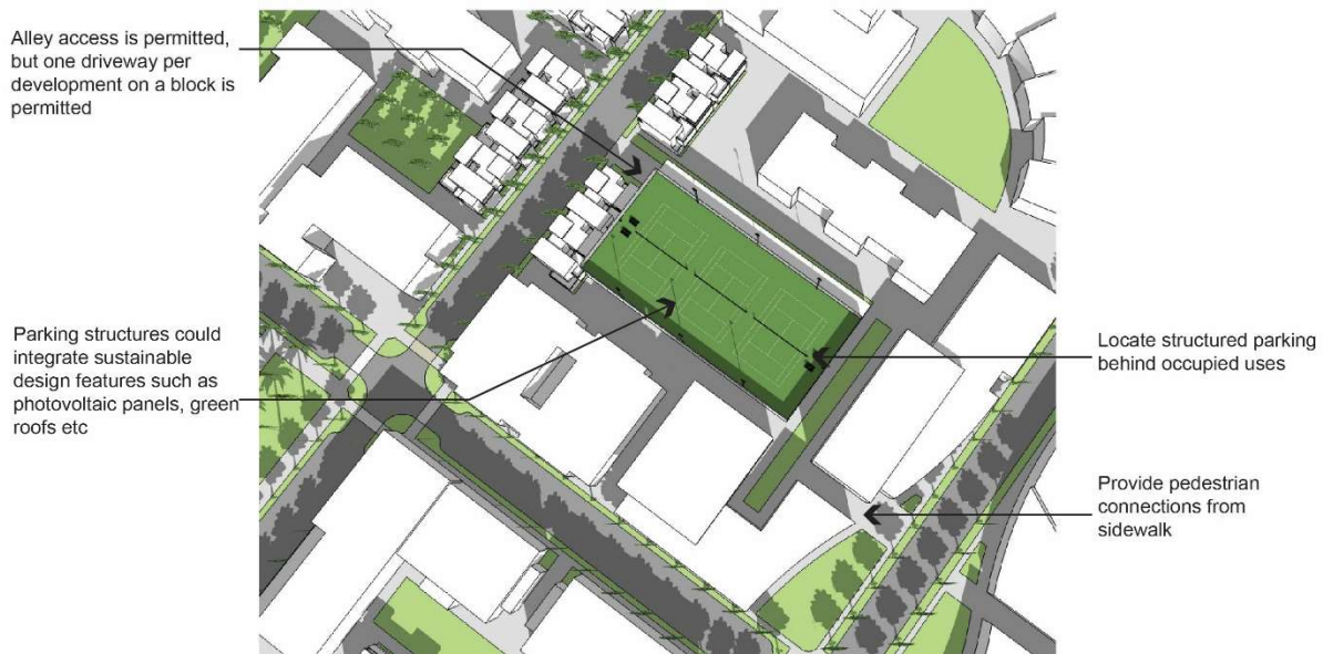
Figure 1-21: Guidelines for parking design in a TOD
